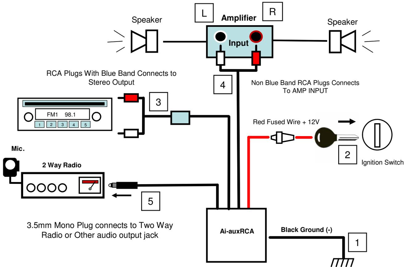
**Ai-auxRCA** is a automatic voice activated mute and switch device that allows seamless interaction between a car stereo and Two Way-Radio. Mounting is out of sight behind the dash. When voice is present (volume set at a pleasant listening level) on a Two Way Radio the Ai-aux RCA automatically switches the audio to Two Way-Radio voice. It remains switched for three seconds after the last voice message is received, then automatically returns back to normal stereo play.
