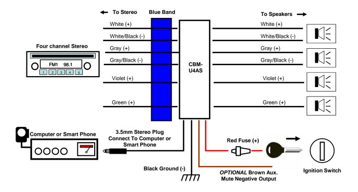
Installing the CBM-U4AS takes only basic wiring skills and tools
