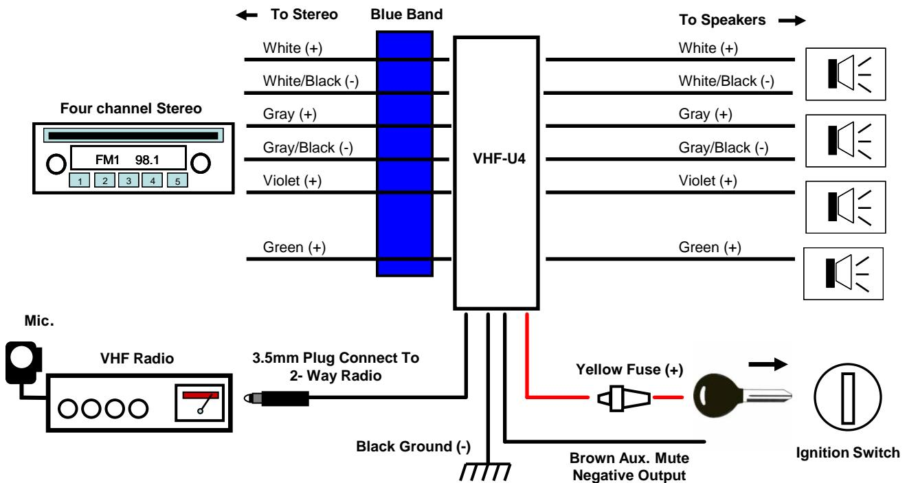
**VHF-U4** is a audio activated, stereo muting and speaker switching device that allows seamless interaction between a marine stereo and a marine VHF 2-way radio equipped with a mono, 1/8" (3.5mm) external speaker, output jack. **Note:** Some VHF, 2-way radios have lead wires for an external speaker output instead of an output jack (see **The 3.5mm** below).
